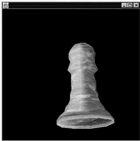
Figure 17 - Chess piece scanned on rotary table rendered with marble texture in JAVA
