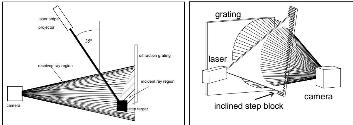
Figure 8 Bench setup with silver halide grating where target is a step block inclined at 10 degrees.
