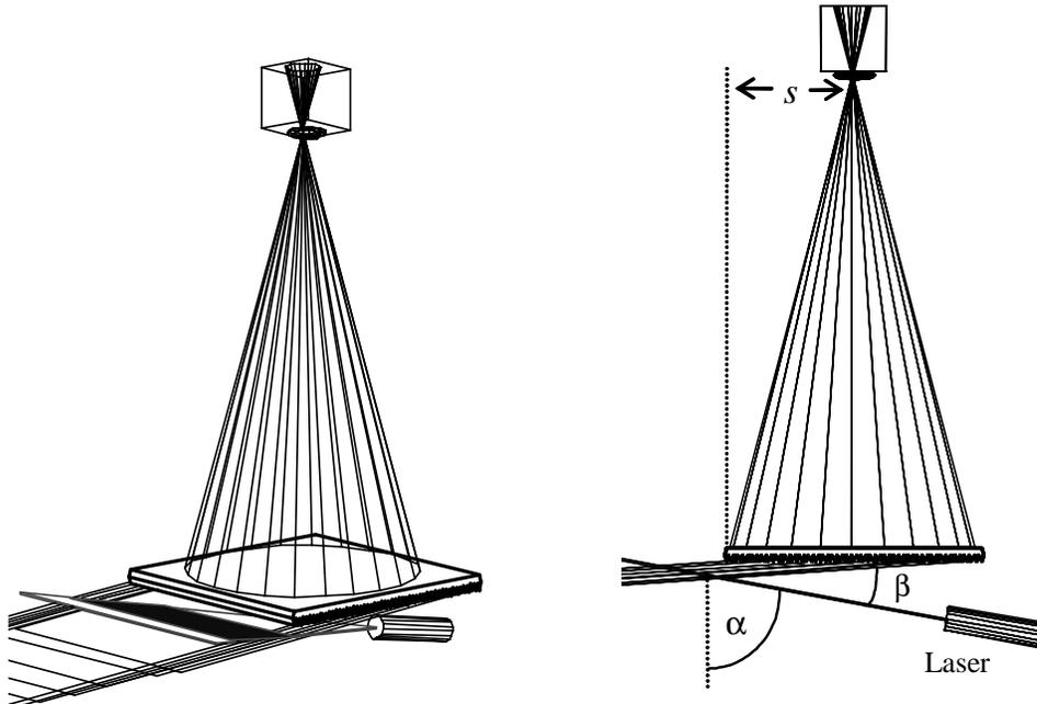
Figure 5 Interrogation of a working volume through the use of a laser projector. The angle of laser  $\alpha$  affects the occlusion liability  $\beta$ . Stand-off  $s$  centers the camera relative to the grating length.
