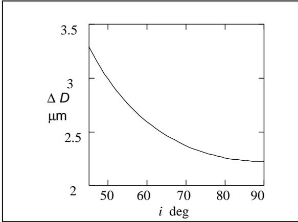
Figure 17 A prediction using a resolving power model Resolution vs. angle of incidence for targets at 10 cm from the grating center.
