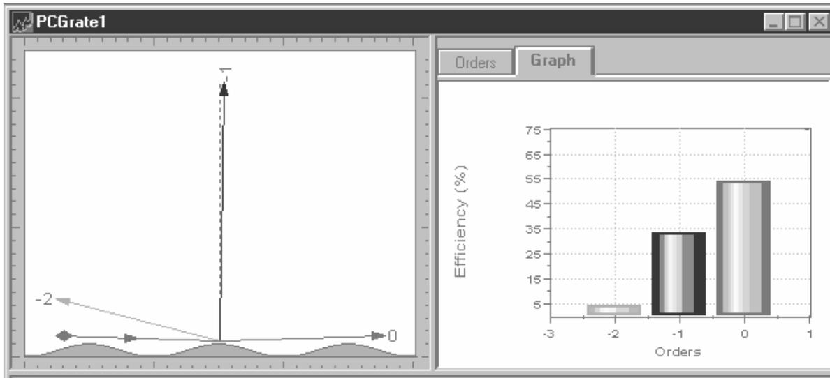
Figure 12 A prediction of PCGrate for  $88^\circ$  grazing incidence is a 35% efficiency in the first-order
