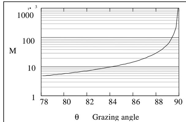
Figure 16 Magnification without concern for diffraction limit. Log scale
