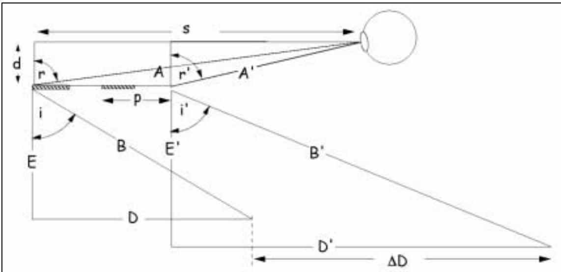
Figure 15 A generalized model for diffraction range finder resolution calculation
