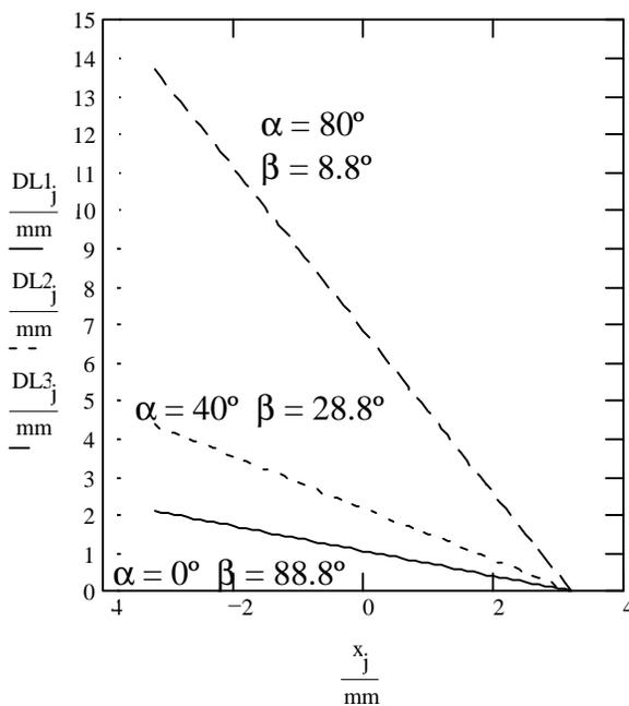
Figure 6 Range vs focal plane displacement for three angles of  $\alpha$  and their correlated occlusion liabilities  $\beta$
