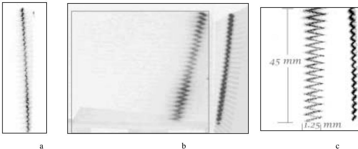
Figure 11 On the left (a) is a triangulation image with an occlusion liability of 20 degrees. The center image (b) is from the same setup but made with the diffraction grating camera. A comparison of the two images in (b) was made with incline removed and annotates the target's actual dimensions (c).
