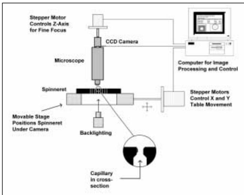
Figure 14 The Aspex SpinTrak<sup>®</sup>, a commercial optical inspection instrument
