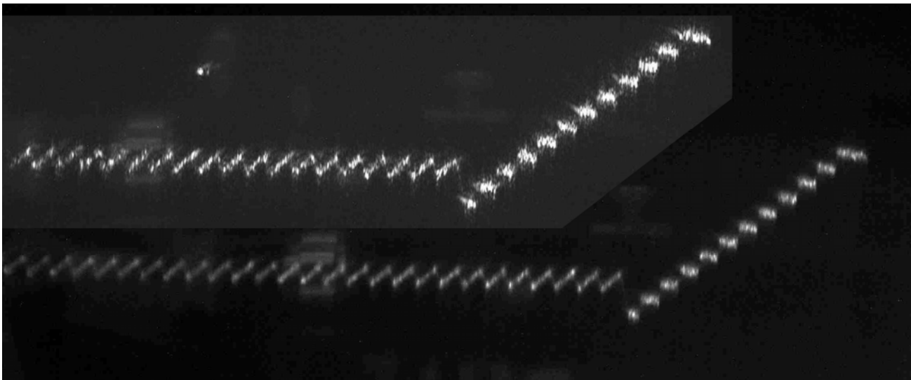
Fig. 10 Eighth inch incremental steps shown with speckle (above) and despeckled (below) sheet of light projection
