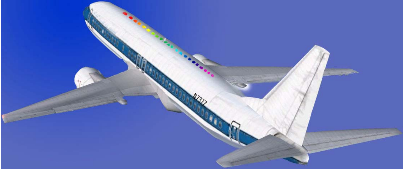
Fig. 10 A concept sketch of the exterior of a transmission POG aircraft. POG segments are placed like windows on the roof.
