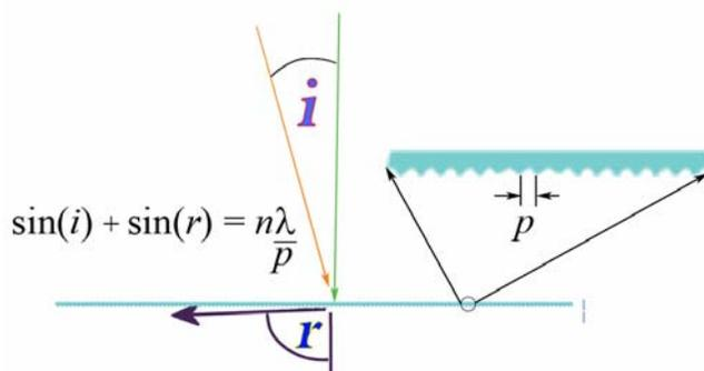
**Figure 3. The Diffraction Equation**
