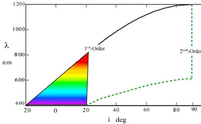
**Figure 4. Free Spectral Range  $p = 600$  nm at  $87^\circ$  grazing**
