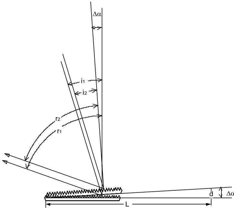
**Figure 10** Parameterization of flatness tolerance specification
