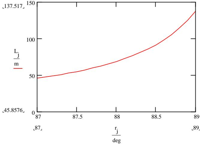
**Figure 7** Length of POG using 2.5 m secondary mirror
