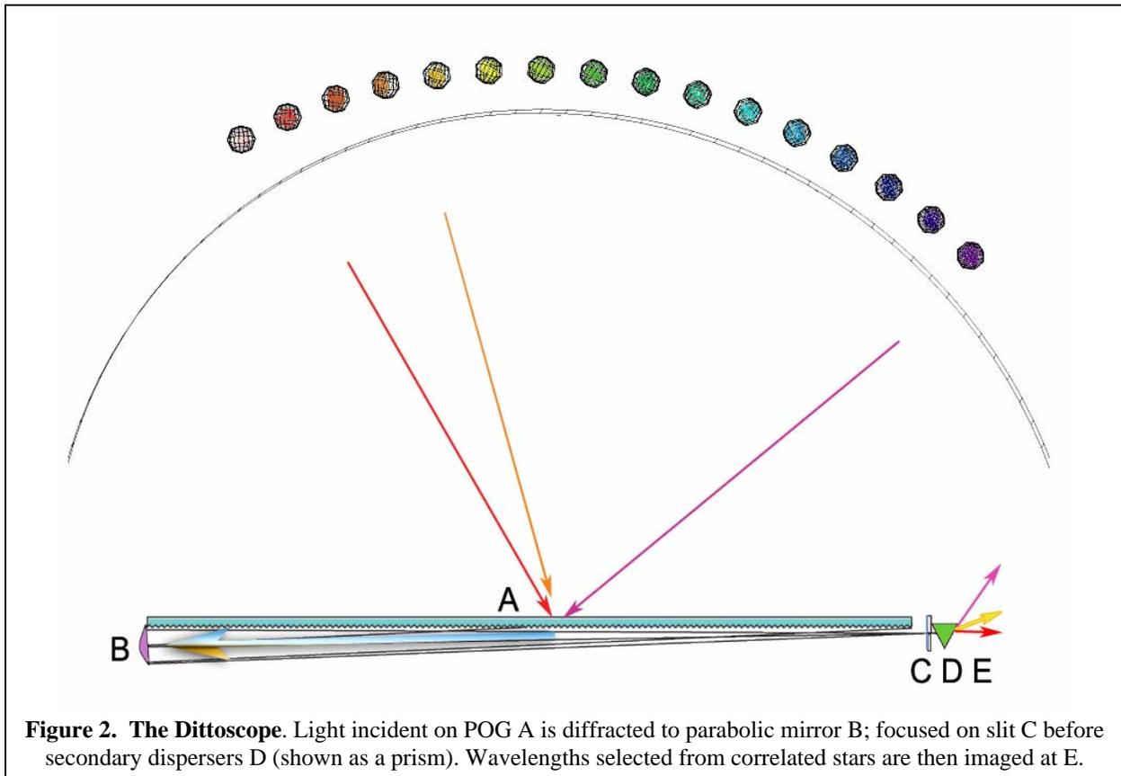
**Figure 2. The Dittoscope.** Light incident on POG A is diffracted to parabolic mirror B; focused on slit C before secondary dispersers D (shown as a prism). Wavelengths selected from correlated stars are then imaged at E.
