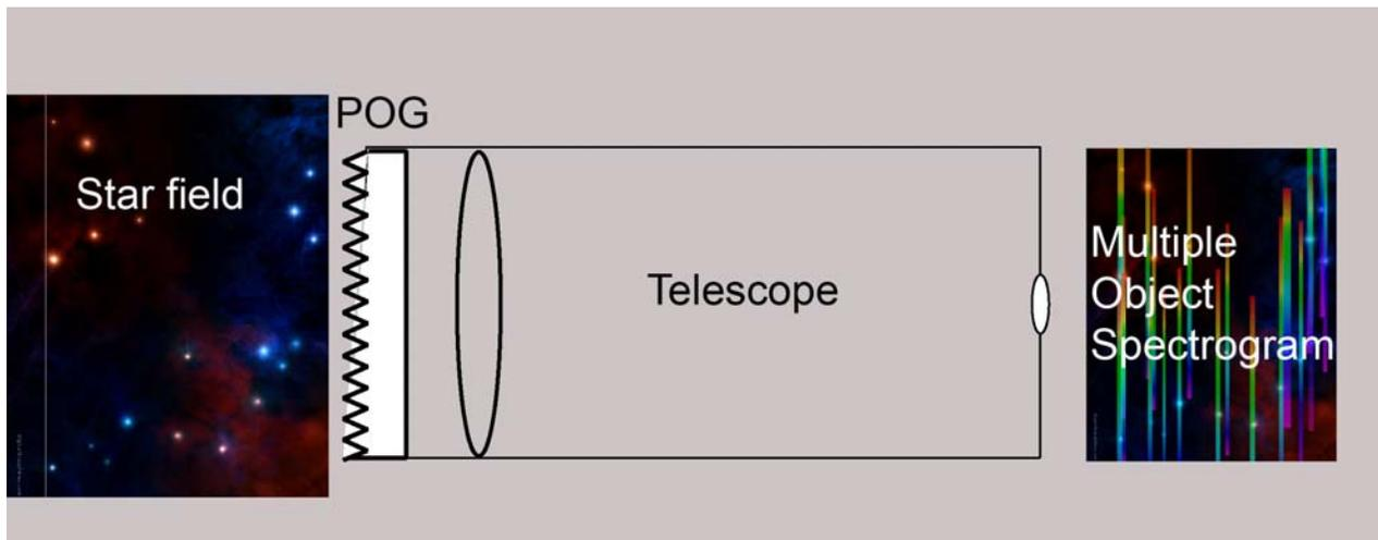
**Figure 1. The Classical Primary Objective Grating Telescope.** The plane grating does not concentrate the flux.
