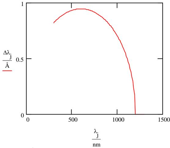
**Figure 11** Ångstrom resolution with garden variety float glass rated at 8 waves per inch supporting a 600 nm grating configured at grazing exodus  $r = 88^\circ$
