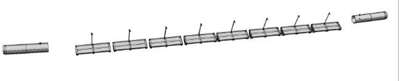
Figure 17 A segmented row of gratings declined for observation with secondary receivers at both extrema .
