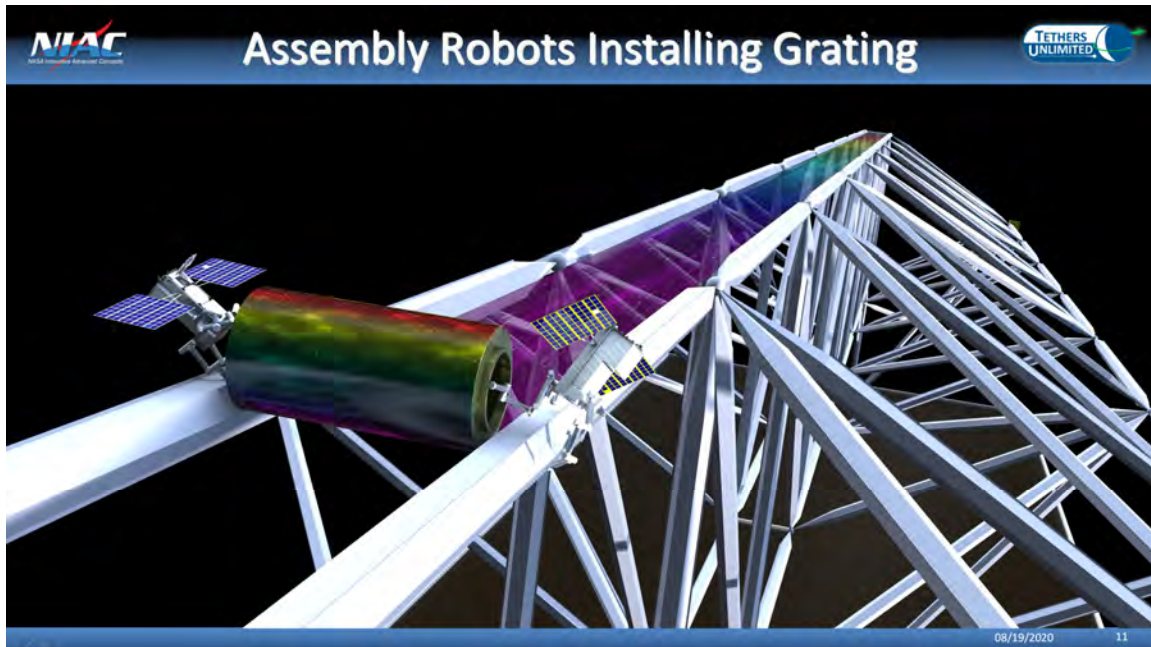
Fig. 5.7 Installation of a 100 m POG from stowed cylinders
