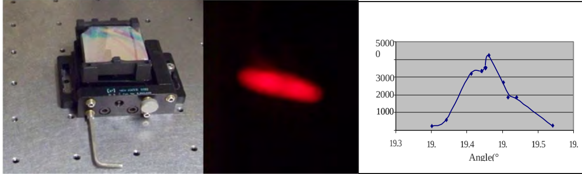
Figure 3.10. Conventionally ruled 4 cm × 4 cm, 1180 line/mm grating ruled on float glass (left). The center image shows the zero-order (reflected) 1 mm spot of a laser, which does not show the caustic patterns seen in Figure 3.9. The right panel shows the shape of the profile of the first-order spot size.
