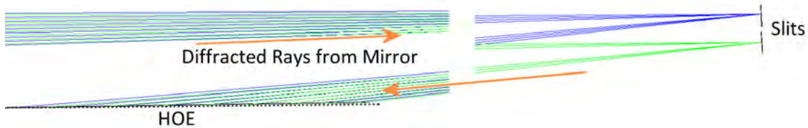
Fig. 5.10 Slit Slats of the Venetian Blind redirecting the same wavelength onto a common secondary HOE
